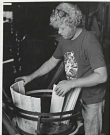
Arranging the staves inside two hoops is an early stage in barrel making.
