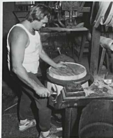
A worker pounds the heading—or circular bottom—on a barrel.
