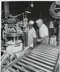
Brooks oversees a late stage, tightening the hoops around a barrel.
