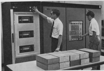
An 1800 data acquisition and control system is used for record keeping as well as the Computer Science course. Pictured are just three parts of the complex computer set-up.
